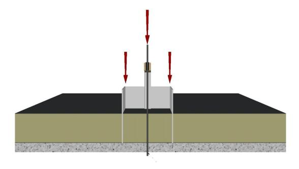
4. Carefully extract the cut insulation from the insulated board and using the pilot hole as a centre point, draw a line which will be located 70mm left and 70mm right and 30mm top and 30mm bottom from the pilot hole.
