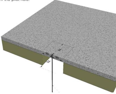
5. Carefully cut the lining board, following the marked lines.
